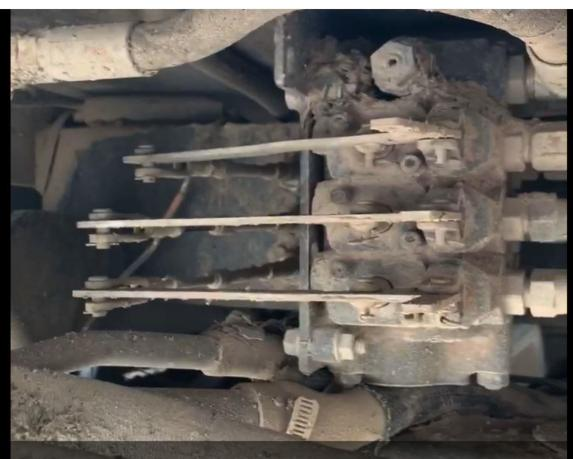
Malfunctioning Pressure Relief cartridge due to debris. Pressure relief would open and close rapidly causing this scenario and the bed would not lift a bale. The solution was to force high flow ratings in pressure relief situations such as the rephase cycle.
